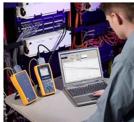
The DTX CableAnalyzer test multiple “victim” links for alien crosstalk during 10 Gigabit/s Ethernet testing. Results are quickly analyzed and stored on a laptop, providing complete documentation of this phase of the 10 GB/s test process.
